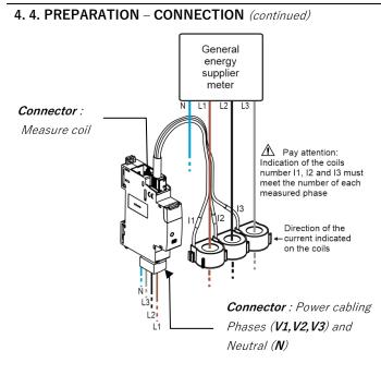
A circuit breaker from C2 to C16 rating is required according to the cable cross section used to supply the three-phases energy meter. The connection between the three-phases energy meter and the coil is made via a connector.
